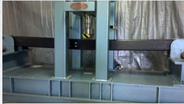
Full Section Testing of SPLICEPLATE
