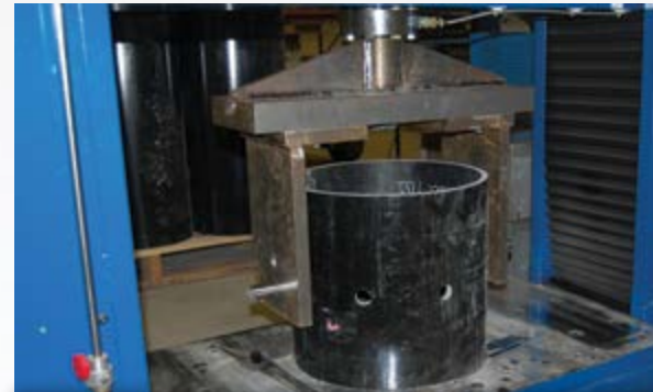
Bolted Connection Test - Parallel
