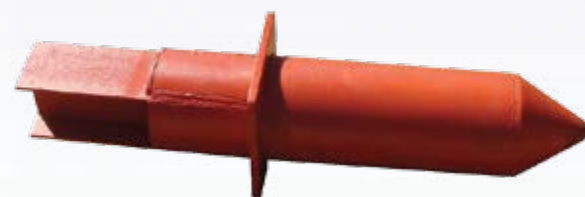
Example of Vibratory Hammer Steel Fabrication
