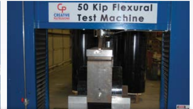
Bolted Connection Test - Perpendicular
