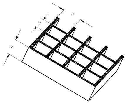
TYPE **D**INLET **N**ON TRAFFIC **F** IBERGLASS MOLDED
